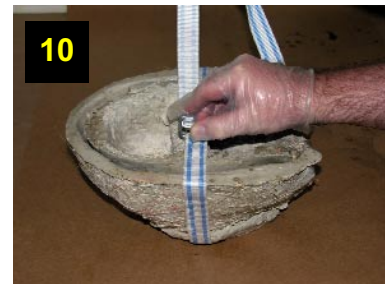
10. As pressure is applied, material is distributed evenly throughout the mold. Dragon Skin and Slacker blend cure for 6 hrs.
