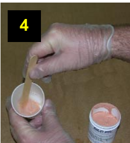
4. Parts A & B are mixed together along with Silc Pig Fleshtone pigment.
