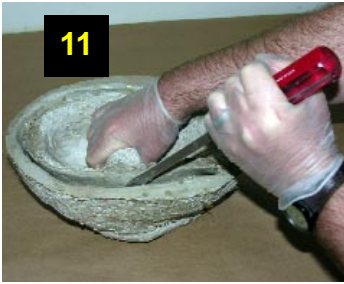
11. The mold strap is removed and a screwdriver is used to break the vacuum that has formed in the mold.
