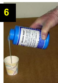
6. Later, one Part A & one Part B of Dragon Skin silicone rubber are then measured out by volume, along with three parts of new Slacker tactile mutator.
