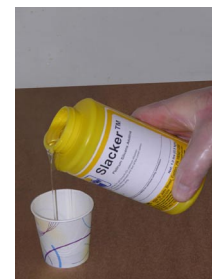
6. Later, one Part A & one Part B of Dragon Skin silicone rubber are then measured out by volume, along with three parts of new Slacker tactile mutator.
