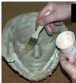
5. The mold cavity and positive face plug are brushed with a thin layer of the skin-tone Dragon Skin silicone rubber. The Dragon Skin layer is cure accelerated with a heat gun in about 5 minutes.
