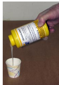
6. Later, one Part A & one Part B of Dragon Skin silicone rubber are then measured out by volume, along with three parts of new Slacker tactile mutator.
