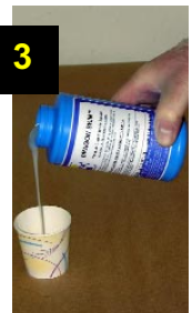
3. Parts A & B of Dragon Skin silicone rubber are measured out 1:1 by volume.
