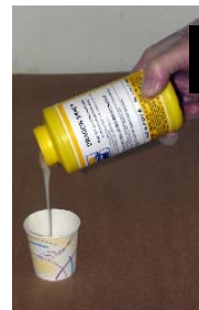
3. Parts A & B of Dragon Skin silicone rubber are measured out 1:1 by volume.
