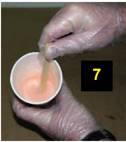
7. The Dragon Skin and Slacker are mixed together along with Silc Pig Flesh tone pigment.
