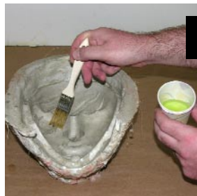
2. The face mold and face plug are coated with the soap/alcohol mixture to release rubber.
