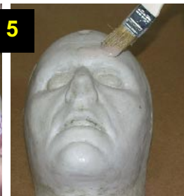
5. The mold cavity and positive face plug are brushed with a thin layer of the skin-tone Dragon Skin silicone rubber. The Dragon Skin layer is cure accelerated with a heat gun in about 5 minutes.
