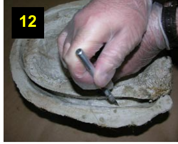
12. An exacto knife is used to cut excess flashing that clings to the mold.
